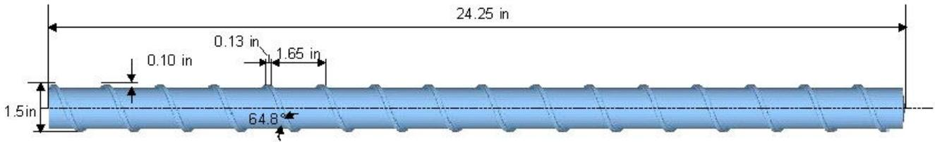
**Figure 1.** A standard cooling screw geometry (Killion's Extruder).
