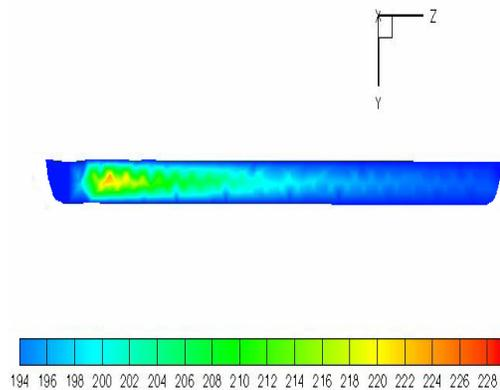
Figure 7. Screw channel cross-section temperature profile
