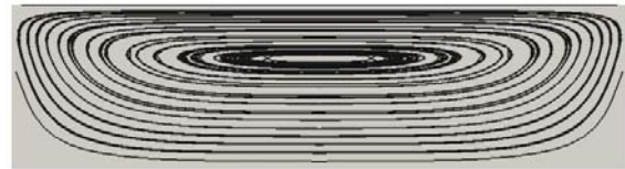
Figure 7. Stream lines of transverse flow. (ST screw)
