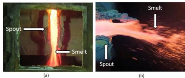
**Figure 2.** A smelt spout viewed (a) from the front, (b) from above. Note that these pictures do not illustrate shattering, as the shatter jets are located somewhat below the spout lip.
