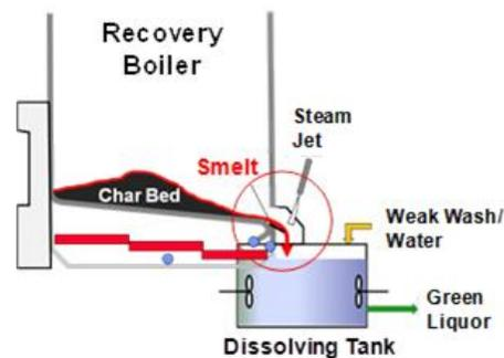
**Figure 1.** A smelt stream from the bottom of the recovery boiler is shattered by a steam jet before falling into the dissolving tank.
