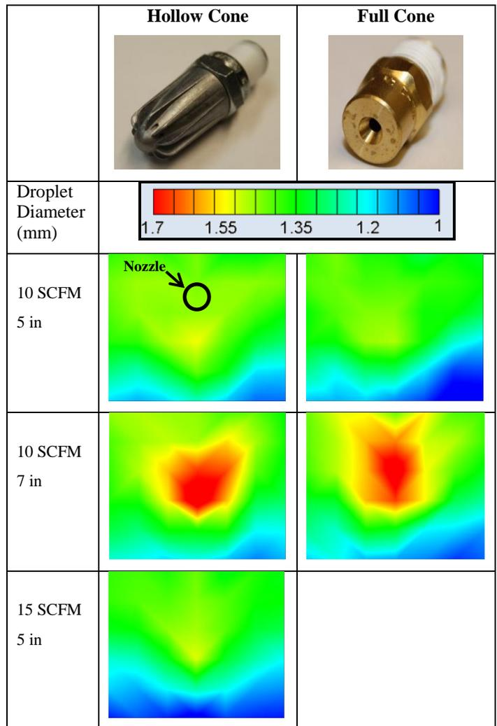
Figure 6(a). Droplet size distributions under various operating conditions. The left column indicates air flow rate and impingement distance. 15 SCFM was not achievable for the full cone nozzle due to excessive pressure.
