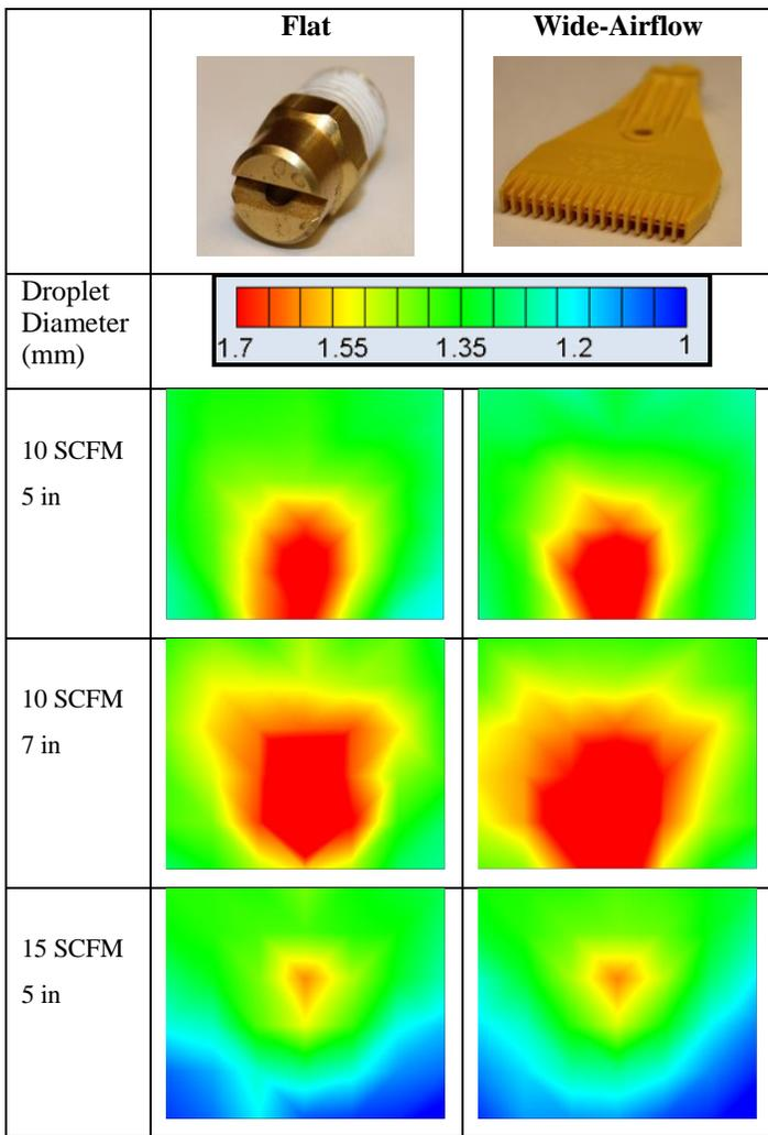
**Figure 6(b).** Droplet size distributions under various operating conditions. The left column indicates air flow rate and impingement distance.
