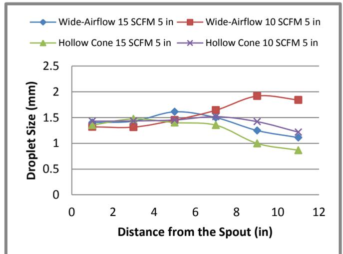
**Figure 8.** Effect of gas flow rate on droplet size distribution. Graph shows centerline average droplet size with respect to the spout.
