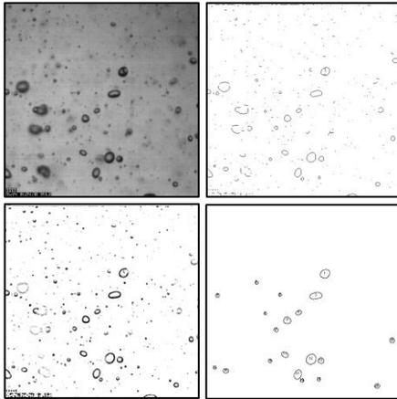
Figure 5: Image processing and analysis using ImageJ™.
