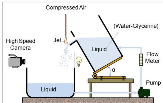
**Figure 3.** Lab scale experimental shattering apparatus.
