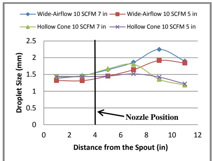
**Figure 7.** Effect of impingement distance on droplet size distribution. Graph shows centerline average droplet size with respect to the spout.
